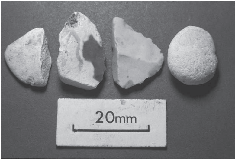
Figure 5.15 Examples of flint and chalk (extreme right) aggregate particles showing the white microporous cortex on the flints (partly broken away on the particle second from left).
