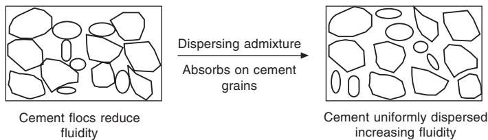
Figure 4.9 Effect of dispersing admixtures in breaking up cement flocs.
