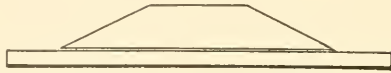
(a) Pat with Top Surface Flattened for Determining Time of Setting by Gillmore Method
