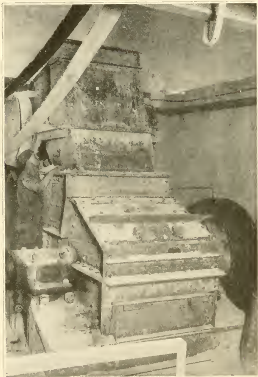
Swinging hammers in the hammer mill batter the rock from the crushers into pieces small enough for the preliminary grinders. The impact sounds like machine-gun fire.
