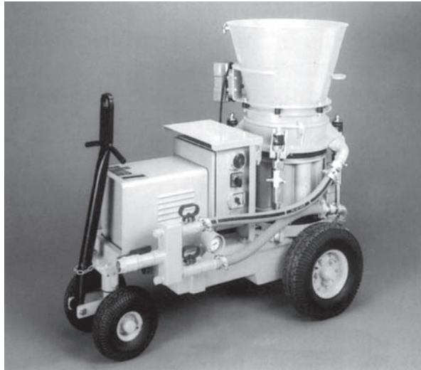
Figure 10.4 Typical dry spray machine (gun).
