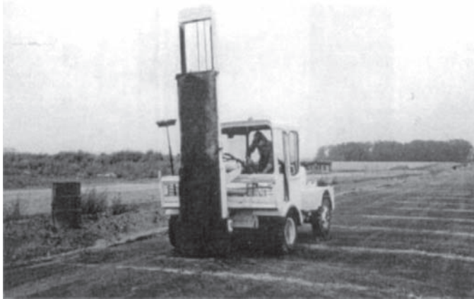
Figure 23.6 A breaker with a heavy blade which could be used to induce cracks in hardened CBM.
