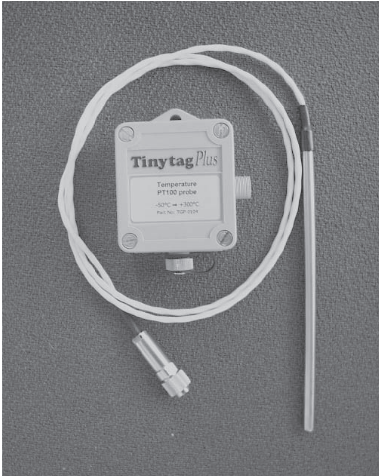
Figure 4.18 Maturity meter (Wexham Development Ltd).
