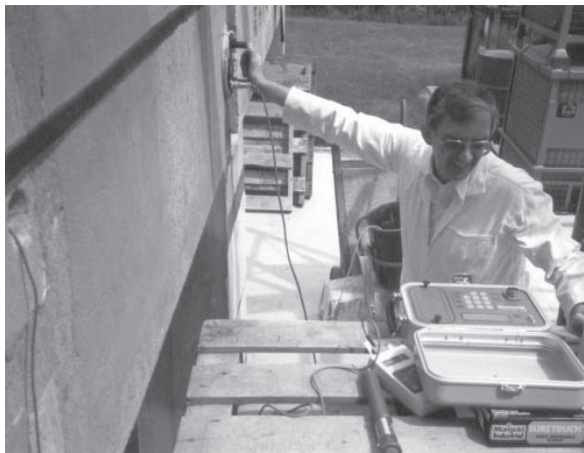
Figure 9.19 A device for measuring the corrosion rate of steel in concrete.
