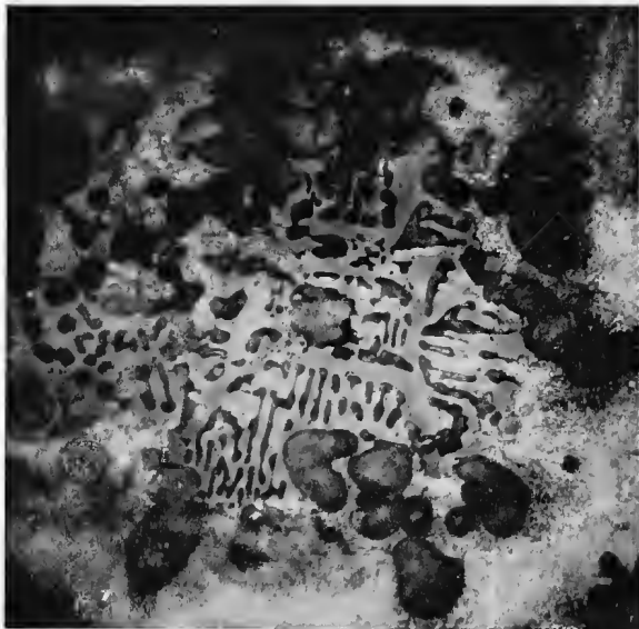
ii. EUTECTIC STRUCTURE IN GRANULATED SLAG. Etched with 1 % HCl. Vertical illumination. \times 300 diam.
