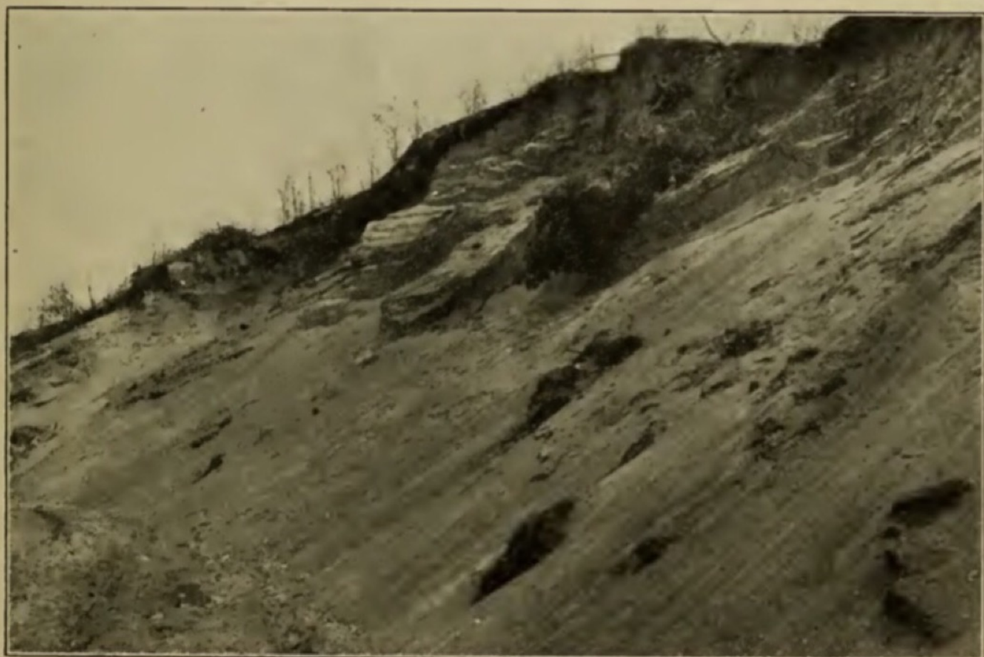
This pit is largely fine material, in addition to which vegetable matter has drifted down across the face of the pit, thus mixing objectionable foreign material with the sand.
